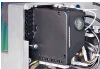
Control box fitted with ignition transformer
